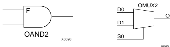
Figure 20: AND & MUX Symbols in XC4000X IOB
